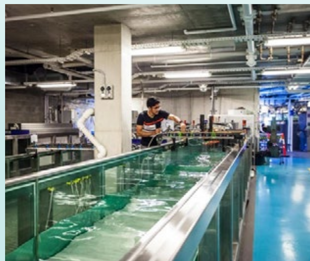
Use of wave flumes to simulate and measure the impact of waves on coral rubble. Image credit: University of Queensland.
